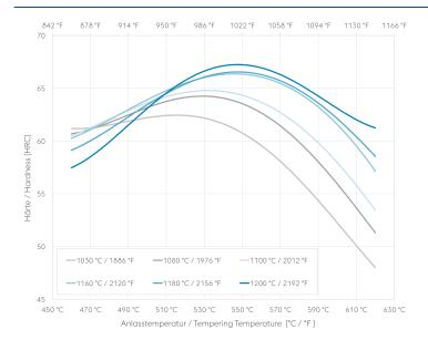
Holding time 3 x 2 hours Specimen size: square 25 mm
