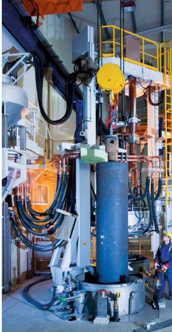
PESR Pressure Electro Slag Remelting
