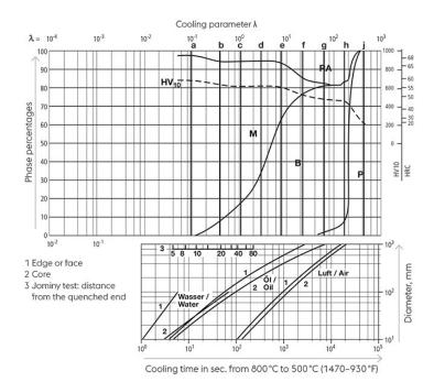
A... Austenite B... Bainite K... Carbide M... Martensite P... Perlite RA... Retained austenite
