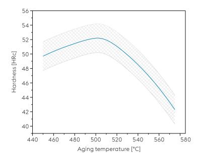
Heat Treatment for optimum properties: Solution Annealing: 1000°C / 1h soaking time / air cooling to room temperature Ageing: 500°C / 3h soaking time / air cooling
