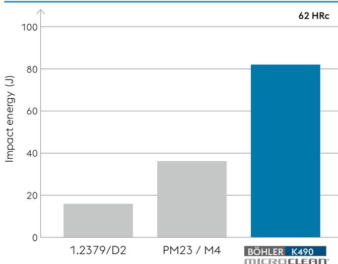
Samples taken from a rolled steel bar in longitudinal direction, heat treated at a cooling rate of:  $\lambda \leq 0.5$
