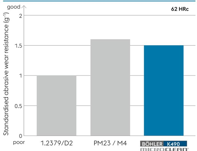
Determined by the rubber disc dry sand test according to ASTM G65
