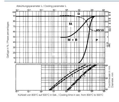
HV10... Vickers Hardness Lk... Ledeburite carbide RA... Residual austenite
