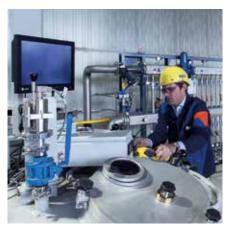
Vacuum induction melting and atomization under inert gas ensure the highest possible metallurgical purity of the powder.
